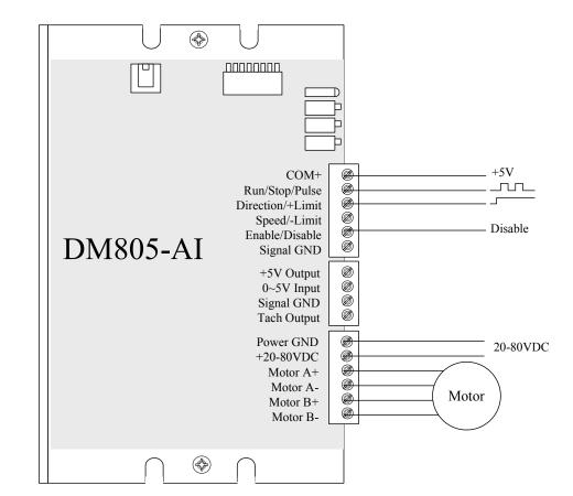
A complete stepping system should include stepping motor, stepping drive, power supply and controller (pulse generator).
